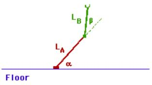
If a specific angle feedback arrives at the controller computer, where is the tool? Using vectors, the tool is at the tip of the resultant vector
