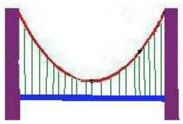
We will presume that the bridge roadbed has uniform linear density  $\beta$  and the wires from cable to roadbed are very numerous and very light in comparison to everything else.
